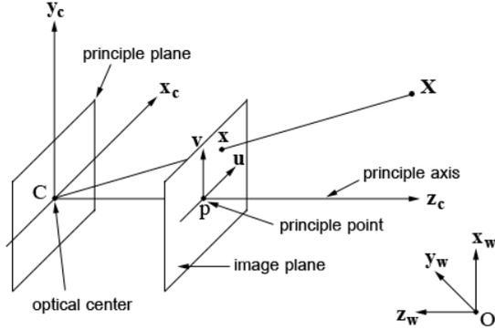
**Fig. 2.** The pinhole camera model.
