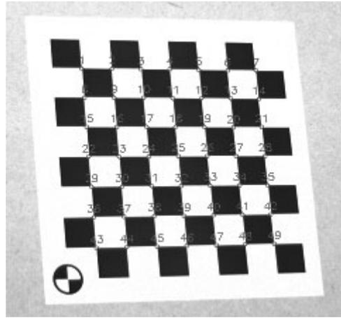
**Fig. 3.** The chessboard pattern for calibration
