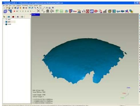
**Fig. 16.** The tri-angular mesh created from the measurement points
