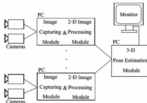
**Fig.1.** An arrangement of the processing modules on PC-cluster.
