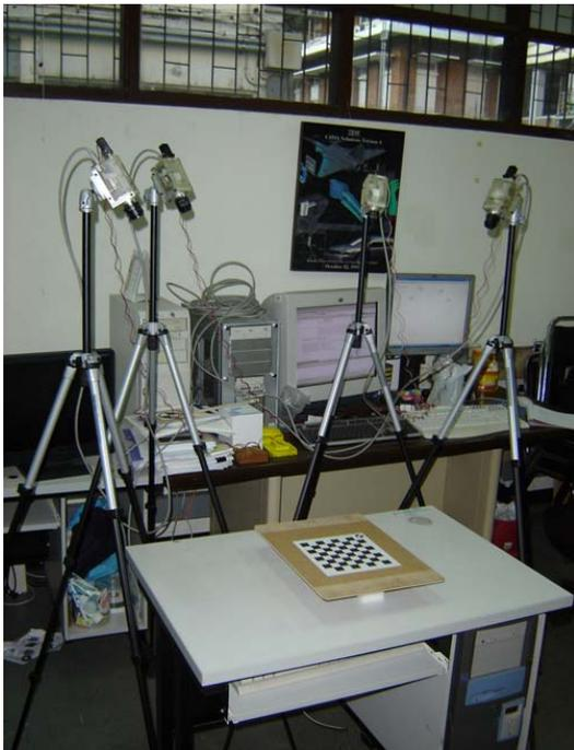
**Fig. 6.** The system setup for testing accuracy of measurements
