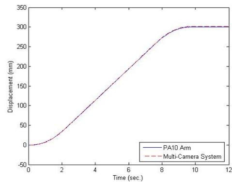
**Fig. 17.** Linear motion with s-curve velocity profile
