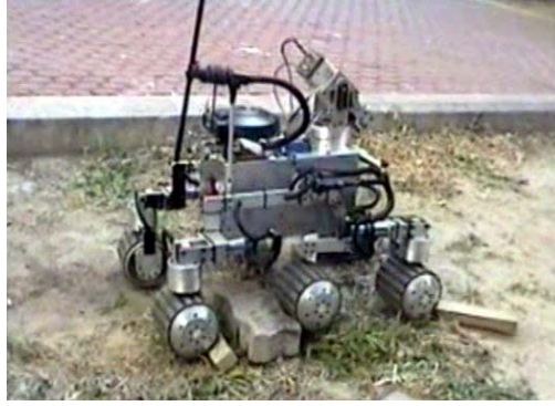
Figure 20: Traversing over obstacles
