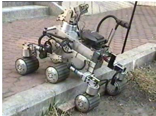
Figure 18: Climbing up a curb
