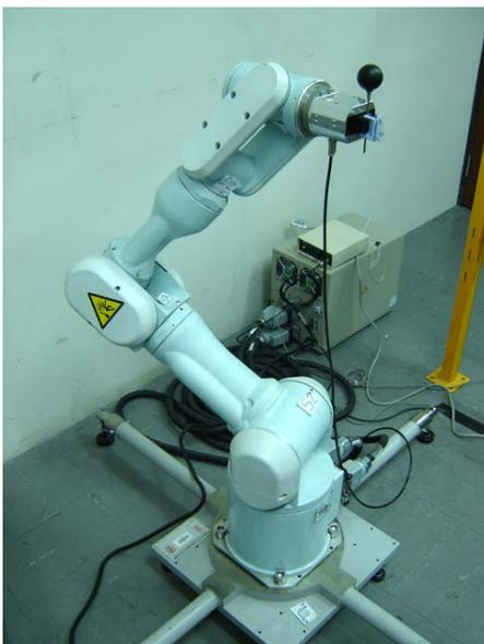
Fig. 8 The robot arm holds a spherical target
