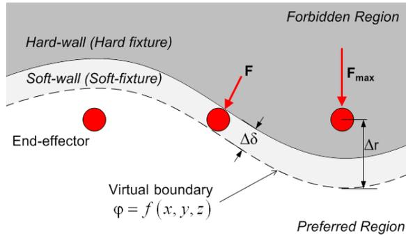
**Figure 5:** Description of a virtual fixture
