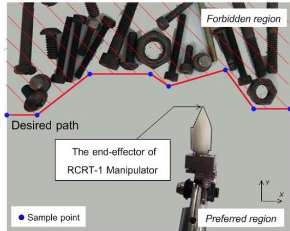
Figure 14: A virtual fixture in the experiment
