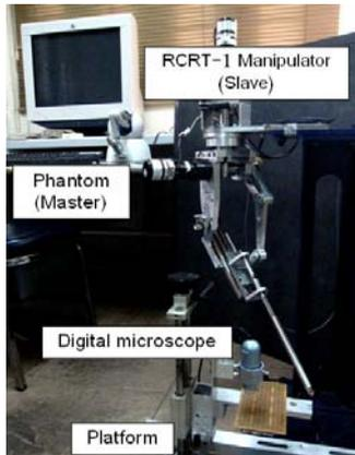
Figure 13: The master-slave system test bed
