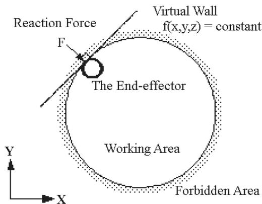
Figure 3: The circular working area
