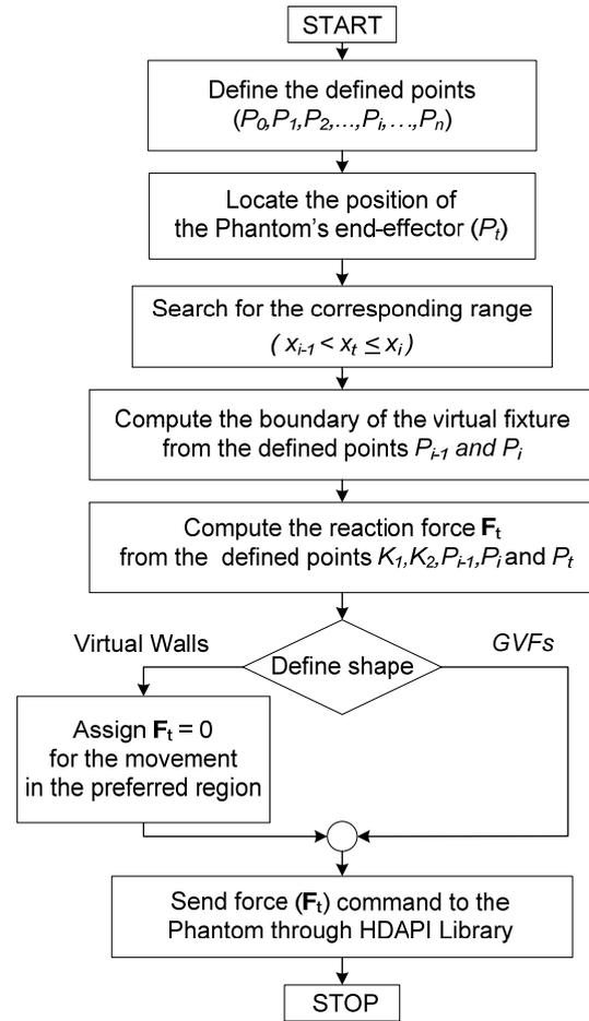
**Figure 12:** Process flowchart of constructing the shape-definable shape virtual fixtures
