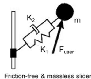
Figure 4: Spring-mass-damper model
