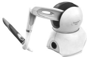
Figure 1: Phantom Omni Haptic Device
