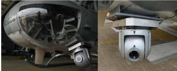
**Figure 6:** The gimbal mounted on the helicopter
